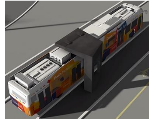
ABB TOSA bus charging system with ultracapacitors
